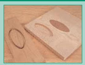
The timber repair template can also be used for inlaying contrasting timbers, veneers or laminates
