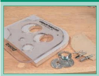
The corner and hole template can be used not only for rounding corners and cutting infinite diameter holes, but for producing accurate, square edged curved templates
